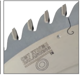
Fig. 2 Example of inspected blade already in perfect balance.
